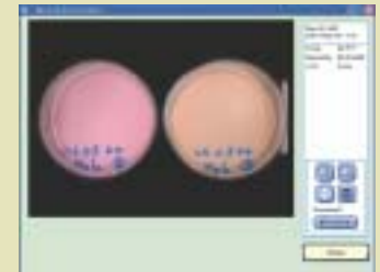
Bird's-eye view image (macro image) Enables you to confirm handwritten vessel notes, change in culture medium color, mold generation, etc.
